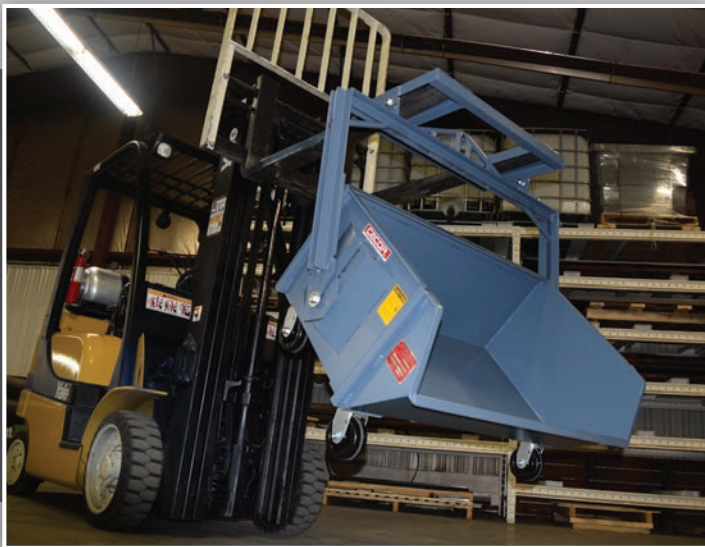
Example of CECOR cart & dumping frame
